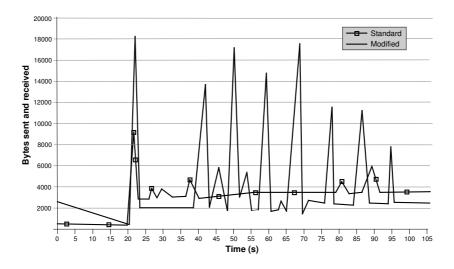
Fig. 4. Average number of overlay maintenance-related bytes per second per host.
